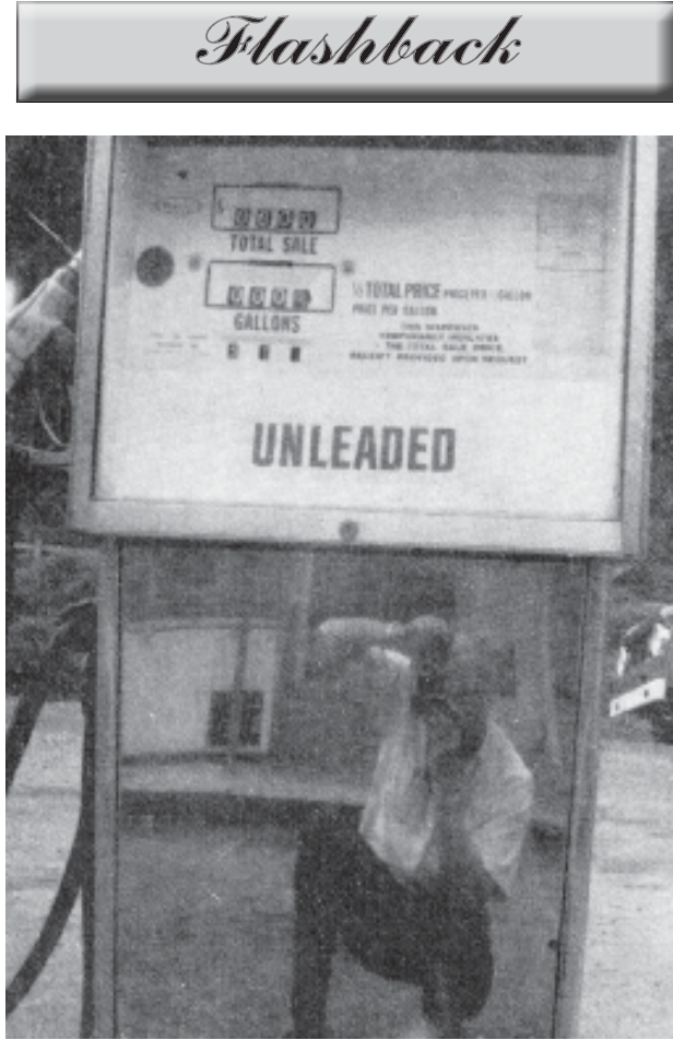
ONLY 51 ¢ FOR GAS, but if you look close you will see that's for a half gallon on this pump, one of many in Snyder County which had to be changed when gas prices went over 99.9¢.
