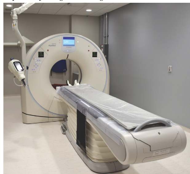
A CT/CTA scanner at the location is a newly purchased model that is state-of-the art and offers shorter scan times, reduced patient dose of radiation, and has improved image quality. The larger bore model improves comfort for patients of larger size or who can experience anxiety while being in tight spaces. For orthopaedic patients the CT CTA technology at the new location offers a metal artifact reduction technique that creates unobscured images during orthopaedic imaging.
